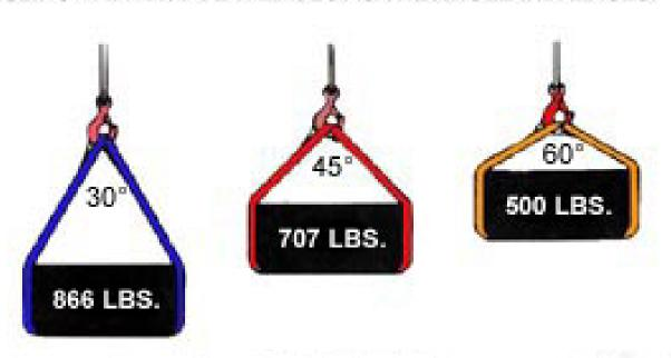
A sling capable of lifting 1000 lbs. in a 30 degree vertical basket hitch, can only lift 866 lbs. at a 30 degree angle, 707 lbs. at a 45 degree angle, and 500 lbs. at a 60 degree angle.
